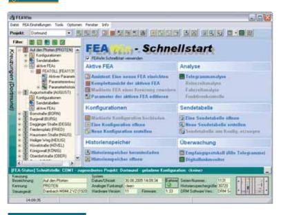
The PC service program FEAWin is used as comprehensive, Windows-based tool, which can be used to manage all FEA functions.
